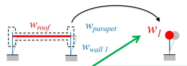
Weight of the building is lumped at the roof level
